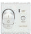
19411.16.B C 16, I_{\Delta n} 10 mA breaking capacity 3000 A - 2 modules. Depth: 39 mm
