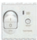
19411.16.6.B C 16, I_{\Delta n} 6 mA breaking capacity 3000 A - 2 modules. Depth: 39 mm
