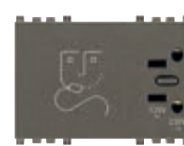
▲19290.M 230 V~ 50/60 Hz, with 20 VA isolating transformer, 230 V~ and 120 V~ outputs - 3 modules. Depth: 41,5 mm
