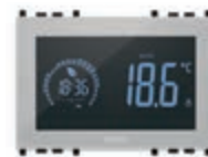
02955.BN Touch screen, ON/OFF and PID temperature control, 1 temperature sensor input, 1 multi-function input, 1 RJ9 input for energy meter (02960), 5(2) A 230 V~ change-over relay output - 3 modules. Depth: 35,3 mm
