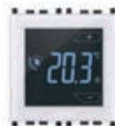
02950.B Touch screen, ON/OFF and PID temperature control, 1 input for temperature sensor, 1 multi-function input, 5(2) A 230 V~ change-over relay output - 2 modules. Depth: 38,5 mm
