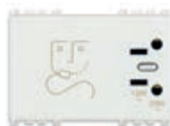
19290.B 230 V~ 50/60 Hz, with 20 VA isolating transformer, 230 V~ and 120 V~ outputs - 3 modules. Depth: 41,5 mm
