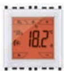
02952.B Touch screen thermostat for ambient temperature control of 2 independent zones, KNX standard, NO 4 A 24 V~ relay output + 1 temperature sensor input + 1 programmable digital input - 2 modules. Depth: 37 mm
