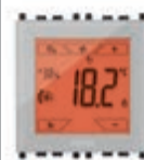
02952.BN Touch screen thermostat for ambient temperature control of 2 independent zones, KNX standard, NO 4 A 24 V~ relay output + 1 temperature sensor input + 1 programmable digital input - 2 modules. Depth: 37 mm
