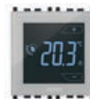
02950.BN Touch screen, ON/OFF and PID temperature control, 1 input for temperature sensor, 1 multi-function input, 5(2) A 230 V~ change-over relay output - 2 modules. Depth: 38,5 mm
