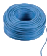
732H.E.100 Due Fili Plus cable for internal laying, 2x1 mm 2 twisted conductors, PVC sheath, CPR Eca class, operating temperature -25/+70 °C, not suitable for running through underground channels, suitable for I category cables (U0 = 400 V), blue - 100 m bundle
