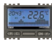
19446.M ON/OFF with input for remote control via dialler, 6(2) A 230 V~ change-over relay output AA (LR6) 1,5 V battery (supplied) - 3 modules. Depth: 42,5 mm
