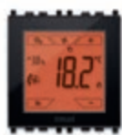
02952 Touch screen thermostat for ambient temperature control of 2 independent zones, KNX standard, NO 4 A 24 V~ relay output + 1 temperature sensor input + 1 programmable digital input - 2 modules. Depth: 37 mm
