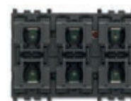
▲01587 6-button + actuator for laths orientation, cosφ 0,6 2 A 120-240 V~ 50/60 Hz change-over relay output - 3 modules Depth: 37 mm
