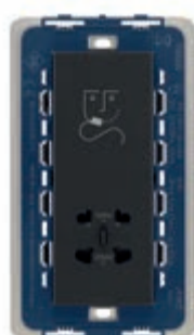
19291 6 230 V~ 50/60 Hz, with 20 VA isolating transformer, 230 V~ and 120 V~ outputs. Depth: 41,5 mm
