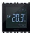
02950 Touch screen, ON/OFF and PID temperature control, 1 input for temperature sensor, 1 multi-function input, 5(2) A 230 V~ change-over relay output - 2 modules. Depth: 38,5 mm
