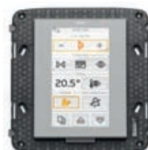
21848.1..M Color touch screen, 4,3", Full Flat, for the control, 1 temperature sensor input, with built-in mounting frame for installation in 8-module mounting box. Depth: 50,4 mm
