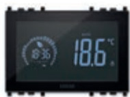
02955 Touch screen, ON/OFF and PID temperature control, 1 temperature sensor input, 1 multi-function input, 1 RJ9 input for energy meter (02960), 5(2) A 230 V~ change-over relay output - 3 modules. Depth: 35,3 mm
