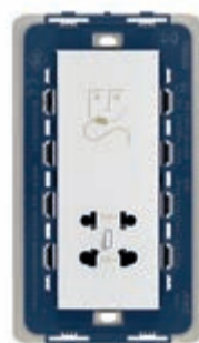
19291.B 6 230 V~ 50/60 Hz, with 20 VA isolating transformer, 230 V~ and 120 V~ outputs. Depth: 41,5 mm
