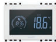
02955.B Touch screen, ON/OFF and PID temperature control, 1 temperature sensor input, 1 multi-function input, 1 RJ9 input for energy meter (02960), 5(2) A 230 V~ change-over relay output - 3 modules. Depth: 35,3 mm
