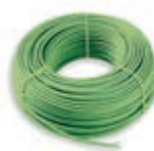
▲01890.C KNX system cable, 2x2x0,8 mm cable, LSZH sheath, CPR Cca s1b d1 a1 class, suitable for I category cables (U0 = 400 V), green - 100 m
