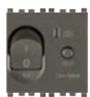
▲19411.06.M C 6, I_{\Delta n} 10 mA breaking capacity 1500 A - 2 modules. Depth: 39 mm
