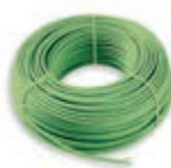
01890.E KNX system cable, 2x2x0,8 mm cable, LSZH sheath, CPR Eca class, suitable for I category cables (U0 = 400 V), green - 100 m
