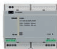
01901 Stereo amplifier, 2 outputs for sound dif- fusers 8 \Omega 10+10 W, power supply 110-230 V~ 50/60 Hz, built-in line terminator, 6 x 17,5 mm modules
