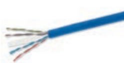
03071.B2 Cat. 6 U/UTP cable, unshielded, 4-pair, 23 AWG, LSZH sheath, CPR B2ca class, blue - 500 m
