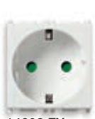
14208.FX SICURY 2P+E 16 A, German - 2 modules. Depth: 32,5 mm
