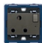
19217.M.5 SICURY 2P+E 15 A, 1-gang, switched. Depth: 25,5 mm
