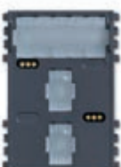
21457.1 Eikon Tactil touch transponder card reader, KNX standard, 2 relay outputs NO 4 A 24 V~, 2 inputs, 12-24V~ 50/60 Hz and 12-24 Vdc (SELV) - 3 modules. Supplied without transponder card. Depth: 36,5 mm
