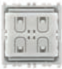
03955 4-button flat device with RF transmission, 868 MHz, EnOcean® standard, energy harvesting supply powered by built-in electrodynamic generator, to complete with buttons - 2 modules. Depth: 3,5 mm
