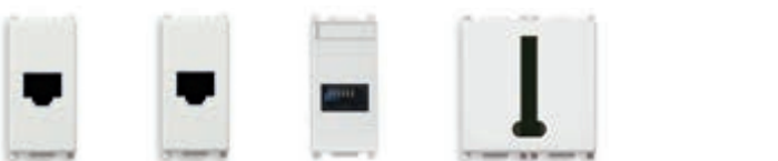
14320 RJ11, 6-position 4-contact (6/4) 14320.AB As above, antibacterial treatment. Depth: 32,4 mm 14321 RJ12, 6-position 6-contact (6/6). Depth: 32,6 mm 14324 Israeli standard, screw terminals. Depth: 32,4 mm 14327 8-contact, French standard - 2 modules. Depth: 21 mm
