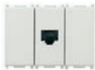
14505.AB Relay module with RJ45 socket outlet for tail call lead with 2 lights + 2 AUX, connection with an 8IN/8OUT module or a Call-way display, 4 24 V NO relay outputs, anti-bacterial treatment - 3 modules. Depth: 29,5 mm
