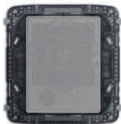
21588.B Passive speaker, 8 Ω 10 W, with built-in 8-module frame. Depth: 48 mm
