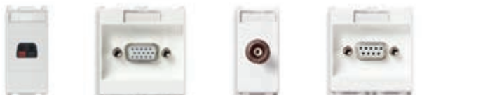
14583 Spring connector for speaker. Depth: 18,4 mm 14348 VGA, 15-pin. Depth: 10 mm Δ 14361 BNC, RG58, RG59/62, RX93 soldering. Depth: 10 mm Δ 14365 9-contact, SUB D, soldering - 2 modules. Depth: 10 mm
