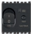
19411.10 C 10, I_{\Delta n} 10 mA breaking capacity 3000 A - 2 modules. Depth: 39 mm
