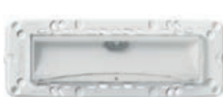
02660.1 With high-efficiency LED, 230 V~ 50/60 Hz, rechargeable Ni-Cd battery and built-in 7-module frame. Depth: 43 mm Δ 02660.1.120 As above, 120 V~. Depth: 43 mm
