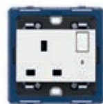
19221.B.4 SICURY 2P+E 13 A, 1-gang, switched. Depth: 17,5 mm
