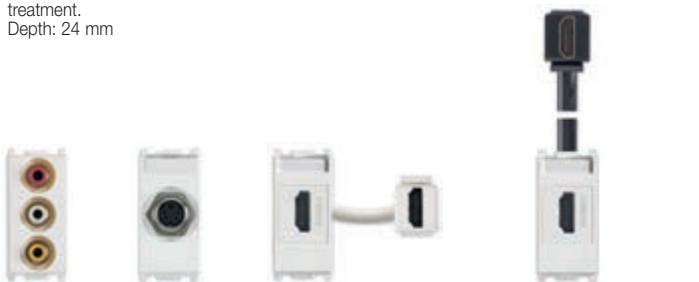
14335 3 RCA outlets, screw terminals. Depth: 23,4 mm Δ 14347 S-Video, 4-pin. Depth: 15,5 mm 14346 HDMI outlet, Keystone connection. Depth: 36,4 mm 14346.H HDMI outlet, Keystone connection, with 90° cable. Depth: 29,4 mm
