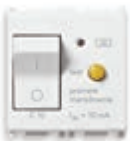
14411.10 C 10, I_{\Delta n} 10 mA breaking capacity 3000 A - 2 modules. Depth: 38 mm
