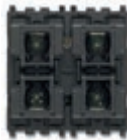
01489 4-button, 1 0/1-10 V SELV output, 1 NO 2 A 120-240 V~ 50/60 Hz relay output for ballast and LED driver, visible in darkness with RGB LED brightness adjustment - 2 modules. Depth: 37 mm
