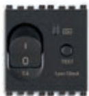
19411.06 C 6, I_{\Delta n} 10 mA breaking capacity 1500 A - 2 modules. Depth: 39 mm
