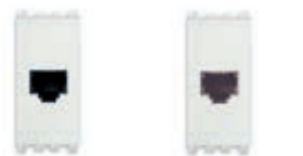
19320.B RJ11, 6-position, 4-contact (6/4). Depth: 33,1 mm 19321.B RJ12, 6-position, 6-contact (6/6). Depth: 33,1 mm
