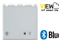
14590.SL 1 4+4 W stereo amplifier, 2 outputs for 8 Ω sound diffusers with built-in Bluetooth ® wireless technology receiver, 1 LINE IN, supply voltage 12 Vdc - 2 modules. Depth: 36 mm
