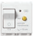
14411.06 C 6, I_{\Delta n} 10 mA breaking capacity 1500 A - 2 modules. Depth: 38 mm
