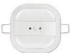
01527 IR presence detector, 360° motion range, ON/OFF and adjustment of lighting, heating, air conditioning, ventilation, 1-1000 Lux adjustable brightness range, KNX standard, for ceiling installation. Dimensions: 80x80x45 mm
