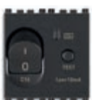
19411.16 C 16, I_{\Delta n} 10 mA breaking capacity 3000 A - 2 modules. Depth: 39 mm
