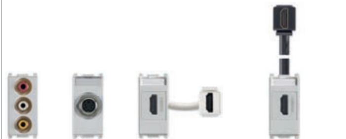
14335.SL 3 RCA outlets, screw terminals. Depth: 23,4 mm Δ 14347.SL S-Video, 4-pin. Depth: 15,5 mm 14346.SL HDMI outlet, Keystone connection. Depth: 36,4 mm 14346.H.SL HDMI outlet, Keystone connection, with 90° cable. Depth: 29,4 mm
