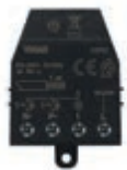
03992 ON/OFF sequence pulse relay module, 1 input for NO push button, 1 input for reset push button, 1 NO 10 A 220-240 V~ 50/60 Hz relay output, luminous signalling of load status, for backfit
