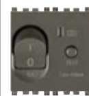
19411.06.M C 6, I_{\Delta n} 10 mA breaking capacity 1500 A - 2 modules. Depth: 39 mm
