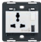
■ 20266.A.B SICURY 2P+E 13 A 250 V~, multistandard, with 1 2P 1-way switch and 1 USB-A. Depth: 21 mm
