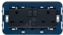
■ 19224.AC SICURY 2P+E 13 A 250 V~ with 2 2P 1-way switches, 1 USB-A and 1 USB-C. Depth: 21 mm
