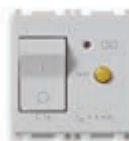
14411.16.6.SL C 16, I_{\Delta n} 6 mA breaking capacity 3000 A - 2 modules. Depth: 38 mm
