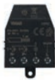
03992 ON/OFF sequence pulse relay module, 1 input for NO push button, 1 input for reset push button, 1 NO 10 A 220-240 V~ 50/60 Hz relay output, luminous signalling of load status, for backfit
