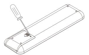
1. Use a right screwdriver to unscrew and remove the screw.
