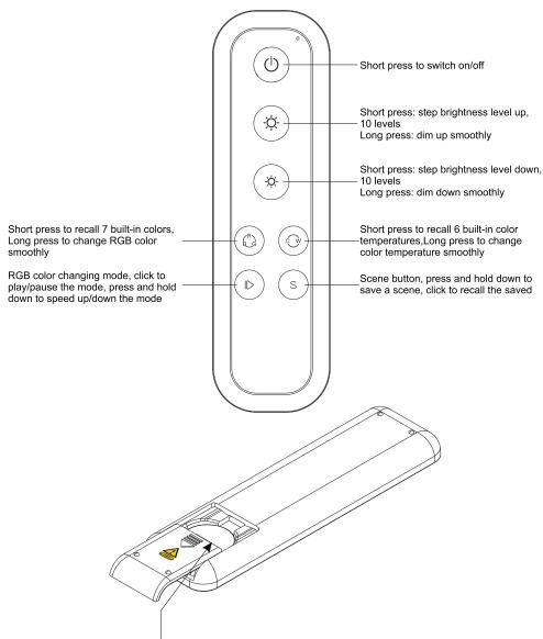
Note: Before the first use, please remove the protective film on the battery.
