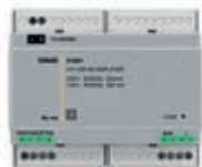
01901 Stereo amplifier, 2 outputs for sound dif- fusers 8 Ω 10+10 W, power supply 110-230 V~ 50/60 Hz, built-in line terminator, 6 x 17,5 mm modules
