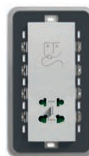
20291.N 6 230 V~ 50/60 Hz, with 20 VA isolating transformer, 230 V~ and 120 V~ outputs. Depth: 41 mm
