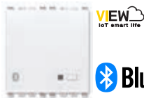
20590.B 1 4+4 W stereo amplifier, 2 outputs for 8 Ω sound diffusers with built-in Bluetooth® wireless technology receiver, 1 LINE IN, supply voltage 12 Vdc - 2 modules. Depth: 36 mm
