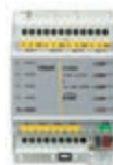
01522 Input/output device, 4 NO 16 A 250 V~ relay outputs, 4 inputs for NO contacts, KNX standard, 4 x 17,5 mm modules
