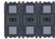
▲21125 8 non-polarised inputs, 7 solid state outputs for non-polarised contacts, 9-32 VDC power supply, for external/internal hotel room or cabin applications - 3 modules. Depth: 22,8 mm
