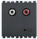
20582 Audio input with 2 RCA connectors, automatic volume adjustment, incorporated line terminator - 2 modules. Depth: 37 mm
