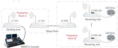
6.3 Extend the communication distance by boost antenna:
