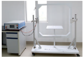
Industrial Frequency Magnetic Field Generation System
