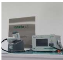
Electrostatic Discharge System
