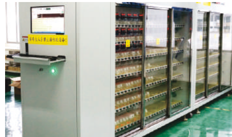
LED Driver Aging Testing Equipment
