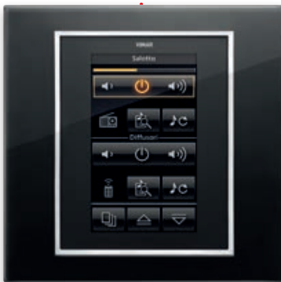
4,3" Full Flat colour touch screen with display of "sound system management" located in the lounge
