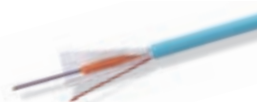
03154.E 50/125 µm OM3 multimodal loose fiber-optic cable, 8-fiber, with LSZH sheath, CPR Eca class, suitable for installation with I Category power supply cables (U0 = 400 V), sea-green - 500 m reel
