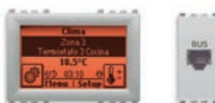
21509.N Control unit for control and configuration, temperature sensor input, supplied with V51923 frame for DIN (60715 TH35) rail installation, 3 modules - Next. Supplied with RJ45 socket connector and V51921 frame. Depth: 37 mm
