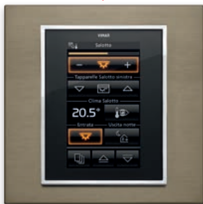
KNX 4.3" Full Flat touch screen for managing automations and climate control.
