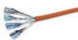
03086.E Cat. 6A S/FTP cable, shielded, 4-pair, 23 AWG, LSZH sheath, CPR Eca class, suitable for I category cables (U0 = 400 V), orange - 500 m
