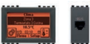
21509 Control unit for control and configuration, temperature sensor input, supplied with V51923 frame for DIN (60715 TH35) rail installation, 3 modules - grey. Supplied with RJ45 socket connector and V51921 frame. Depth: 37 mm
