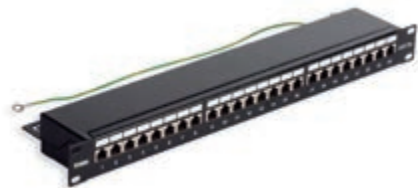
03024.5 24 RJ45 connectors Cat. 5e, shielded, T568A/B universal wiring, 8 contacts, insulation-piercing terminals 110 compatible - 1 rack unit
