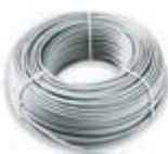
01841.E Bus system cable, 2x0,50 mm 2 , shielded, with LSZH sheath, CPR Eca class, suitable for I category cables (U0 = 400 V), for marine application, white - 100 m
