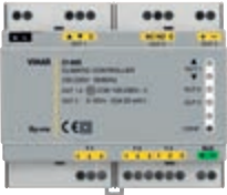
01465 Climate control device for heating systems, power supply 120-230 V~ 50/60 Hz, 3 inputs for PT100, PT1000 and NTC probes, 1 mixer valve control output, 1 0-10 V or (0) 4-20 mA output, 1 16 A 230 V~ change-over relay output, 6 x 17,5 mm modules
