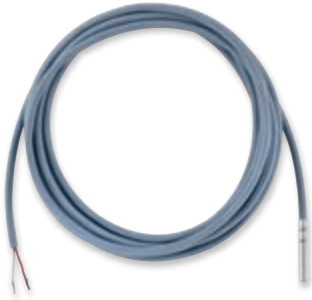
02965.1 Temperature sensor, NTC 10 kΩ, operating temperature -40 °C / +120 °C, IP67, 3 m cable length
