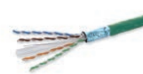
03076.E Cat. 6, F/UTP, 4 pairs, 23 AWG, with LSZH jacket, CPR Eca class, suitable for I category cables (U0 = 400 V), green - 500 m
