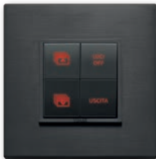
By-me universal home automation control 01480 to control roller shutters and scenarios. The top left push button raises all the roller shutters while the bottom left push button lowers them; the top right push button switches off all the lights and the bottom right one activates the scenario with all lights off and the roller shutters down.
