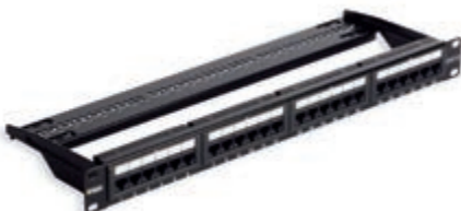
03024.6 24 RJ45 connectors Cat. 6, unshielded, T568A/B universal wiring, 8 contacts, insulation-piercing terminals 110 compatible - 1 rack unit
