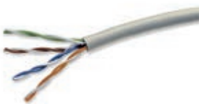
03050.E Cat. 5e, U/UTP, 4 pairs, 24 AWG, with PVC jacket, CPR Eca class, suitable for I category cables (U0 = 400 V), grey - 305 m
