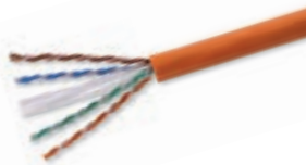
03081.E Cat. 6A, U/UTP, 4 pairs, 23 AWG, with LSZH jacket, CPR Eca class, suitable for I category cables (U0 = 400 V), orange - 500 m
