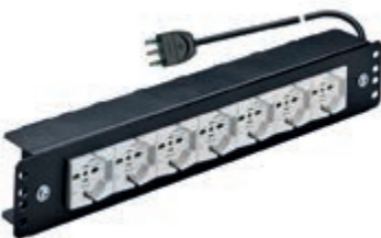
03260 Complete with: • 7 SICURY outlets 2P+E 16 A 250 V~ universal, for Europlugs 2P 2,5 A, plugs 2P and 2P+E 10 A and 16 A Italian standard, plugs 2P+E 16 A 250 V~ German standard, plugs 2P 15 A 125 V~ American standard flat pin, non-polarised. Do not make the earth connection with the 2P+E 16 A 250 V~ French standard plug • 3 m cable 3G1,5 mm 2 and plug S17
