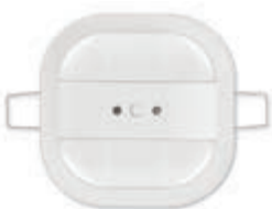
01527 IR presence detector, 360° motion range, ON/OFF and adjustment of lighting, heating, air conditioning, ventilation, 1-1000 Lux adjustable brightness range, KNX standard, for ceiling installation. Dimensions: 80x80x45 mm
