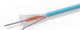
03155.E 50/125 µm OM3 multimodal loose fiber-optic cable, 12-fiber, with LSZH sheath, CPR Eca class, suitable for installation with I Category power supply cables (U0 = 400 V), sea-green - 500 m reel
