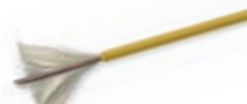
03148.E 9/125 µm OS2 (G.657.A2) monomodal loose fiber-optic cable, 8-fiber, with LSZH sheath, CPR Eca class, suitable for installation with I Category power supply cables (U0 = 400 V), yellow - 500 m reel
