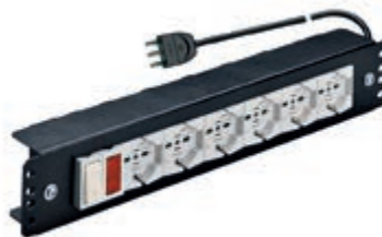
03261 Complete with: • 6 SICURY outlets 2P+E 16 A 250 V~ universal, for Europlugs 2P 2,5 A, plugs 2P and 2P+E 10 A and 16 A Italian standard, plugs 2P+E 16 A 250 V~ German standard, plugs 2P 15 A 125 V~ American standard flat pin, non-polarised. Do not make the earth connection with the 2P+E 16 A 250 V~ French standard plug. • 2P switch • pilot light • 3 m cable 3G1,5 mm 2 and plug S17
