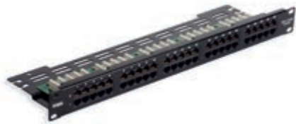
03024.3 50 RJ45 connectors for telephony, insulation-piercing terminals 110 compatible - 1 rack unit
