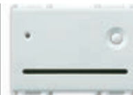
14461 Smart card reader/programmer, 12-24 V~50/60 Hz and 12-24 Vdc (SELV), white - 3 modules. Provided without smart card. Depth: 36 mm
