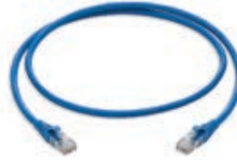
03019.05 RJ45 Cat. 6, U/UTP, 4 pairs, 24 AWG, PVC jacket, blue - 0,5 m
