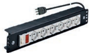
03262 Complete with: • 6 UNIVERSAL SICURY outlets 2P+E 16 A 250 V~, for Europlugs 2P 2,5 A, plugs 2P and 2P+E 10 A and 16 A Italian standard, plugs 2P+E 16 A 250 V~ German standard, plugs 2P 15 A 125 V~ American standard flat pin, non-polarised. Do not make the earth connection with the 2P+E 16 A 250 V~ French standard plug. • circuit breaker 1P+N C 16 • pilot light • 3 m cable 3G1,5 mm 2 and plug S17
