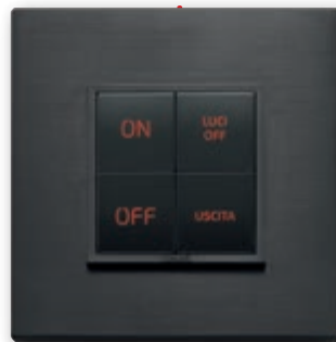
By-me universal home automation control 01481 for controlling lights and roller shutters. The top left push button activates the on-board relay to control a light while the bottom left push button deactivates it; the top right push button switches off all the lights and the bottom right one activates the scenario with all lights off and the roller shutters down.
