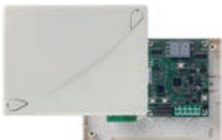
01729 Two-way 868 MHz radiofrequency interface
