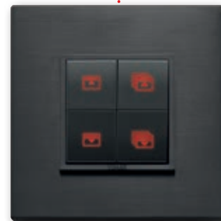
By-me universal home automation control 01482 for controlling slat roller shutters. A long press on the top left push button raises a roller shutter and a long press on the bottom left push button lowers it; the top right push button raises all the roller shutters and the bottom right one lowers them.
