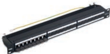
03024.7 24 RJ45 connectors Cat. 6, shielded, T568A/B universal wiring, 8 contacts, insulation-piercing terminals 110 compatible - 1 rack unit
