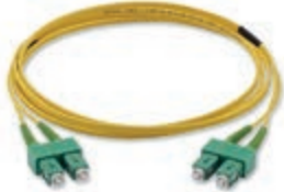
03113.SC Patch cord from SC/APC to SC/APC, 9/125 µm OS2 duplex monomode fibre-optic cable, with LSZH jacket - 2 m
