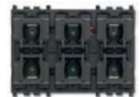
01587 6-button + actuator for laths orientation, with relay output for cosφ 0,6 2 A 120-240 V~ 50/60 Hz motor - 3 modules. Depth: 37 mm
