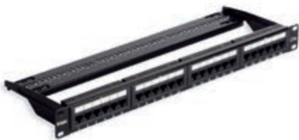
03024.4 24 RJ45 connectors Cat. 5e, unshielded, 568A/B universal wiring, 8 contacts, insulation-piercing terminals 110 compatible - 1 rack unit
