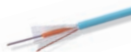
03153.E 50/125 µm OM3 multimodal loose fiber-optic cable, 4-fiber, with LSZH sheath, CPR Eca class, suitable for installation with I Category power supply cables (U0 = 400 V), sea-green - 500 m reel
