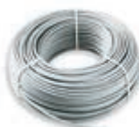
01840.E Bus system cable, 2x0,50 mm 2 , with LSZH sheath, CPR Eca class, suitable for I category cables (U0 = 400 V), white - 100 m
