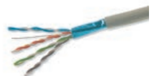
03061.E Cat. 5e, F/UTP, 4 pairs, 24 AWG, with LSZH jacket, CPR Eca class, suitable for I category cables (U0 = 400 V), grey - 305 m
