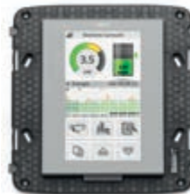
21511.1.BN 4,3" Full Flat, for control, temperature sensor input, with built-in 8-module mounting frame, neutral. Depth: 39,9 mm
