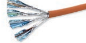
03086.E Cat. 6A, S/FTP, 4 pairs, 23 AWG, with LSZH jacket, CPR Eca class, suitable for I category cables (U0 = 400 V), orange - 500 m
