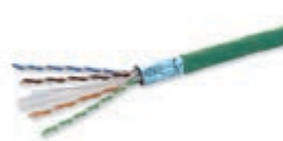
03076.E Cat. 6 F/UTP cable, shielded, 4-pair, 23 AWG, LSZH sheath, CPR Eca class, suitable for I category cables (U0 = 400 V), green - 500 m
