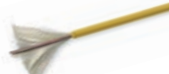
03149.E 9/125 µm OS2 (G.657.A2) monomodal loose fiber-optic cable, 12-fiber, with LSZH sheath, CPR Eca class, suitable for installation with I Category power supply cables (U0 = 400 V), yellow - 500 m reel
